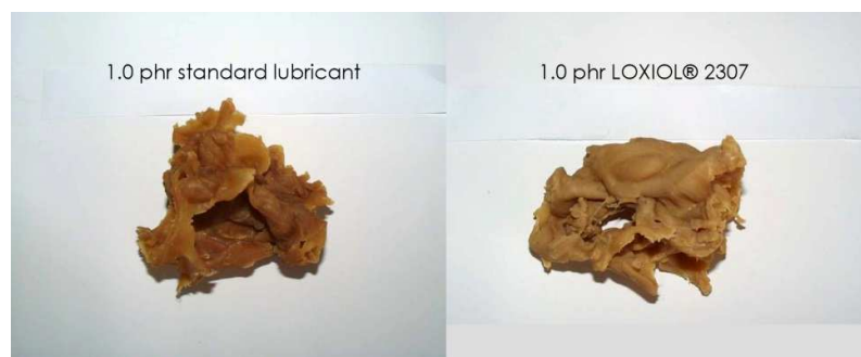
Figure 1: LOXIOI® 2307 (right image) improves dynamic heat stability better than standard lubricant (left image).
