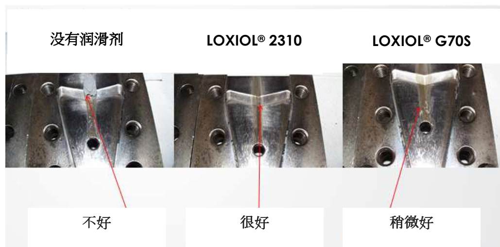
Figure 2: Comparison of plate-out performance without (left image) and with 0.3 phr LOXIOI® 2307 (middle image) and LOXIOI® G 70S after 40 minutes extrusion.
